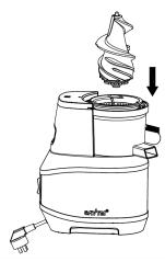
4. Align the triangle on the lid with the unlock mark on the juice container, then clockwise rotate it,
