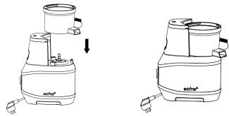
2. Install filter components (the triangle mark on the filter must be aligned with the one on the juice container)
