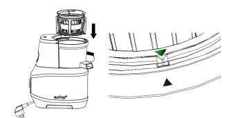
Arrow is at the top of the filter holder, the arrow is relatively small, look for it carefully.
