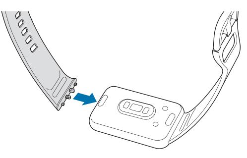
2 Gently pull on both sides of the band to make sure it is tightly connected and not detached from your Fit.
