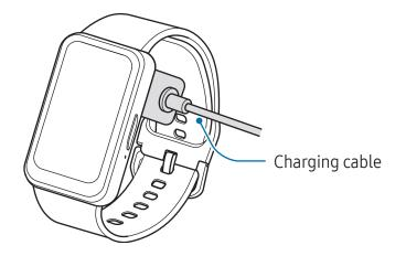
**3** After fully charging, disconnect the Fit from the charging cable.
